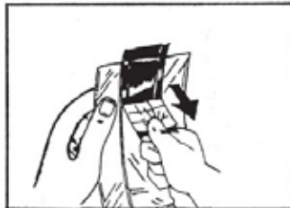
Step 2: Remove the protective paper of the inner sealing tape that will be in contact with the cables while unrolling the product.
