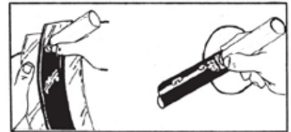
Step 3: Lubricate abundantly the part of the cable jacket which is in contact with the MaxBag and the interior and exterior mastic sealing on bag.
