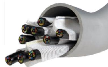
\*\* Use of OFNR cable may result in reduced pulling lengths. Designers should make every effort to conform to industry standards with regard to distances between any two pull points (generally 600 to 1,000 ft), number of bends (maximum of two 90° bends or a total of 180°) between any two pull points, and proofing of conduit pathway using appropriately sized mandrels (normally 1/4" to 1/2" less than the inside diameter of the conduit).
