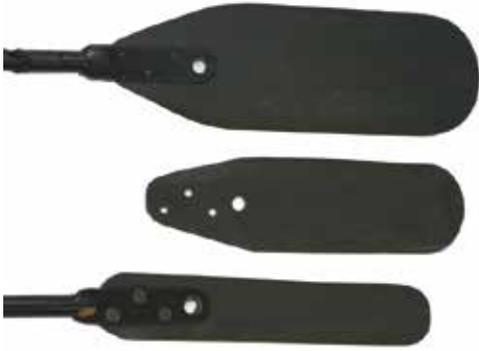
A MaxCell Rodder Head or “paddle” is the most effective tool for overriding existing cable plant. Insertion of the paddle over the top of existing cables presses the cables down in the conduit, creating a larger open space at the top for the placement of MaxCell and subsequent additional cable. The correct size of the Rodder Head selected for any application depends on several factors, including:
